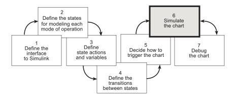
In phase 6 of this workflow, you *simulate the chart* to test its behavior. During simulation, you can *animate* Stateflow charts to highlight states and transitions as they execute.
