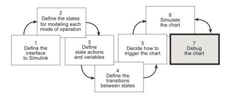
In phase 7 of this workflow, you *debug the chart*. In "Setting Simulation Parameters and Breakpoints", you learned how to set breakpoints and watch data. In this chapter, you will learn how Stateflow software detects errors and provides diagnostic assistance.
