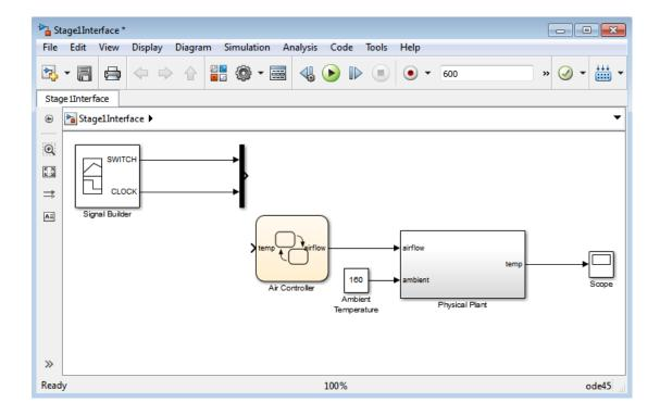
**Tip** You can use a shortcut for automatically connecting blocks. Select the source block, and then hold down the **Ctrl** key and left-click the destination block.
