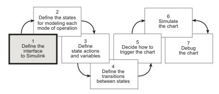
In phase 1 of this workflow, you define the interface to the Simulink model.
