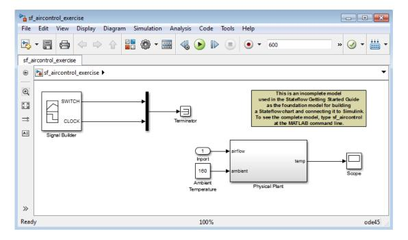
The model is incomplete because it does not include the Stateflow chart that you will build as you work through the exercises in this guide. Instead, the model contains several nonfunctional blocks: the Terminator, Inport, and Annotation blocks.
