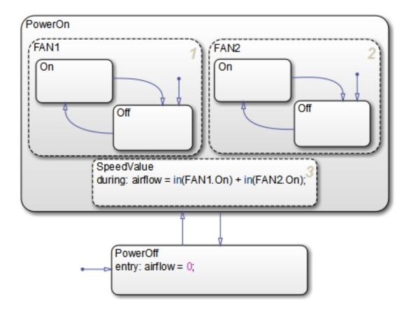
**Tip** The location of the tail of a default transition determines the state it activates. Therefore, make sure that your default transition fits completely inside the parent of the state that it activates. In the Air Controller chart pictured above, notice that the default transition for FAN1.Off correctly resides inside the parent state, FAN1. Now consider this chart:
