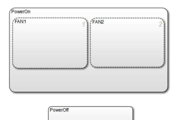
**Note** Your chart might not show the same execution order for parallel substates FAN1 and FAN2. The reason is that, by default, Stateflow software orders parallel states based on order of creation. If you add FAN2 before FAN1 in your chart, FAN2 moves to the top of the order. You will fine-tune order of activation in a later exercise, "Setting Explicit Ordering of Parallel States" on page 4-12.
