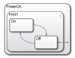
In this example, the tail of the default transition resides in PowerOn, not in FAN1. Therefore, it will activate FAN1 instead of FAN1.Off.
